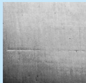
研磨圧力高すぎによる研磨キズ残存 Scratch remains due to overload.
